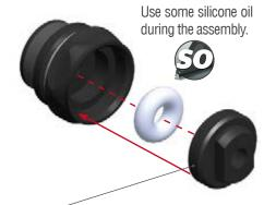
Completely tighten the nut, once the pistonshaft is inserted (step 31.1).
